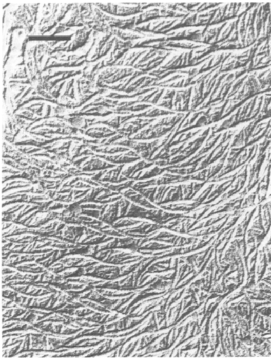
Figure 6 Magnification of similar area to those marked "S" in Fig. 5. The quenched material takes the form of S-shaped sheets. The scale bar = 250 nm. T_c = 124^\circ\text{C} for 10 h.
