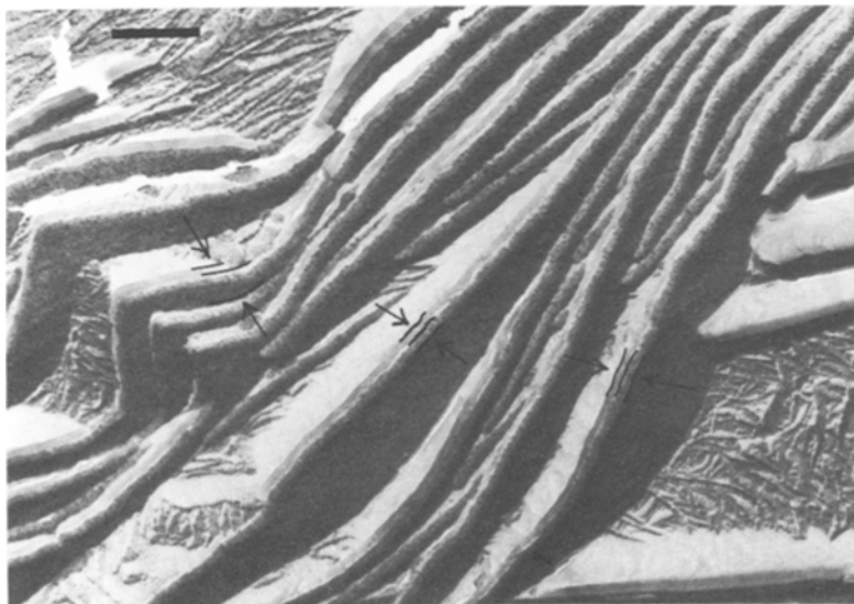
Figure 9 Doublet appearance of isothermally grown thick lamellae. Scale bar = 125 nm. T_c = 124^\circ \text{C} for 40 h.
