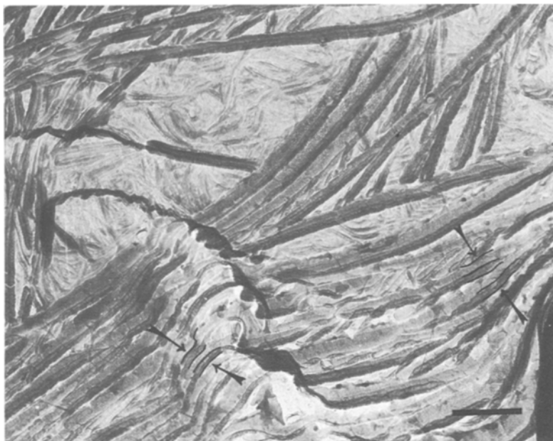
Figure 10 Contrast variations showing fine lamellar features; doublets and triplets. Scale bar = 1 \mu\text{m} . T_c = 124^\circ\text{C} for 30 h.
