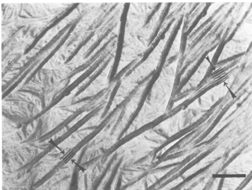
Figure 11 Contrast variations showing fine lamellar features; doublets and triplets. Scale bar = 1 \mu\text{m} . T_c = 124^\circ\text{C} for 30 h.
