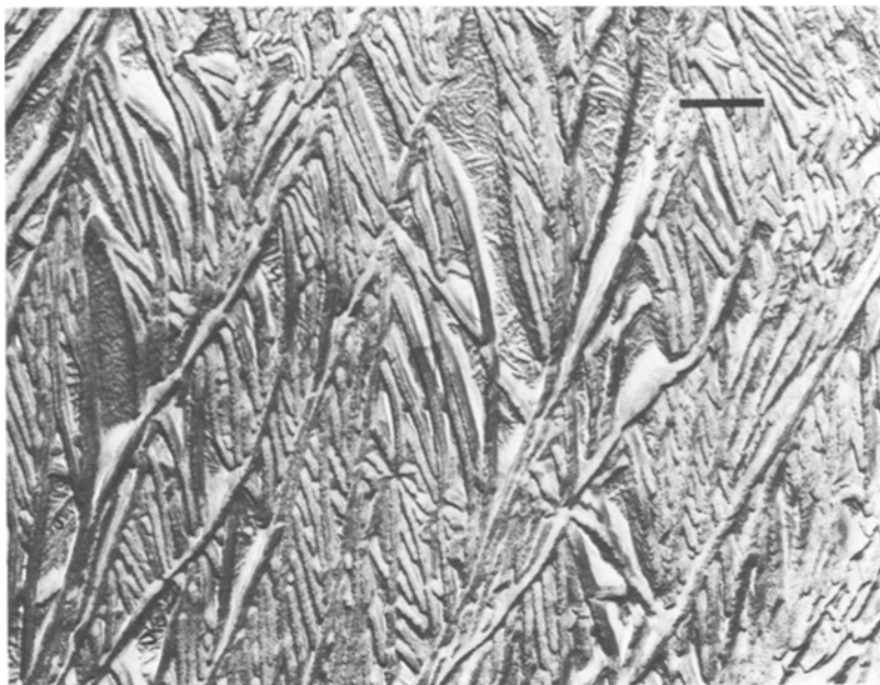
Figure 8 Highly complex composite of the two phases within a spherulite. Quenched material is marked S. Scale bar = 500 nm. T_c = 124^\circ \text{C} for 50 h.
